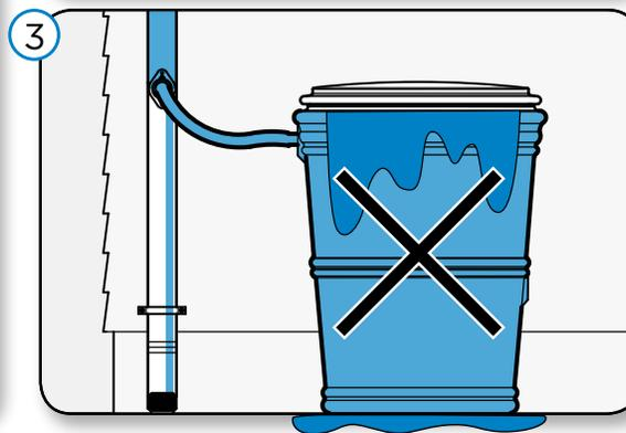
If the hole is cut too low, the barrel will not fill.
